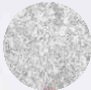
LARGE GRAIN CARBIDE SIZE: ≤ 4.8 µm
